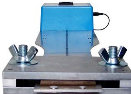
Depress and hold the calibration pushbutton located on the side of the display enclosure with the point of a pen or end of a paper clip for a minimum of 6 sec, the calibration LED will begin to slowly flash green.
