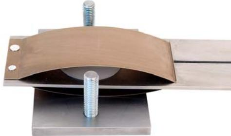
Place the .250" Calibration Plate over the upper spring with guide pins aligned in the holes. Install a washer and wing nut on each guide pin.
