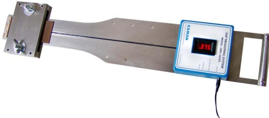
While pushing down on the .375" Calibration Plate, tighten the wing nuts until the Calibration plate is firmly seated on the Base Plate. Check to make sure both of the legs on the Calibration Plate are in full contact with the Base Plate.
