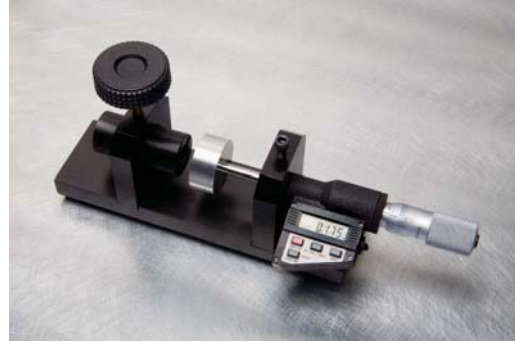
Micrometer calibration fixture.
