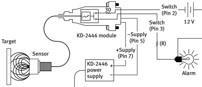
Figure 5. Output is +5V when a gear tooth is seen by the sensor.
