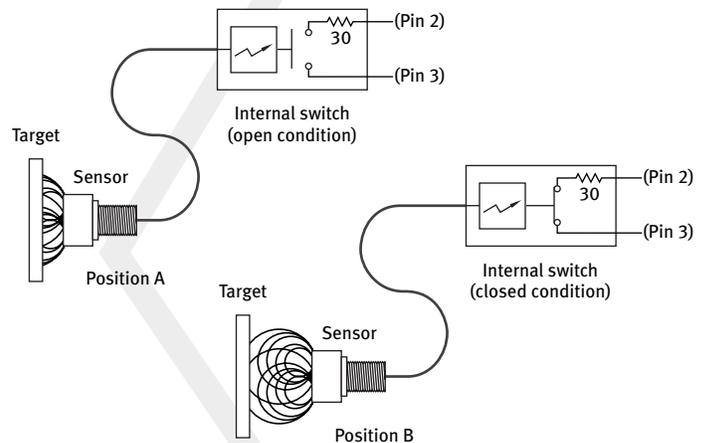
Figure 3. The switch closes and completes the circuit when the sensor-target displacement reaches point B.
