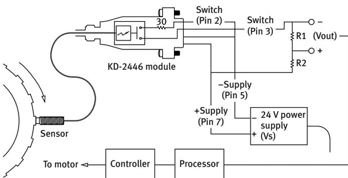
The KD-2446 may also be used to obtain specific output voltages across the switched output connections. This may be done using an external power supply or the supply used to power the KD-2446 module. A simple voltage divider network may be used to calculate a specific output voltage, based on the available input power supply voltage as in the following examples.
